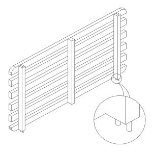
4. Insert the mattress base into the most appropriate mattress height on the cot sides
